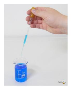
Pipettes must always be held vertically and the solution only transferred short distances.
